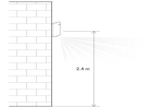
Installing the detector at any other height will narrow the detection zone, affecting the quality of motion detection.
